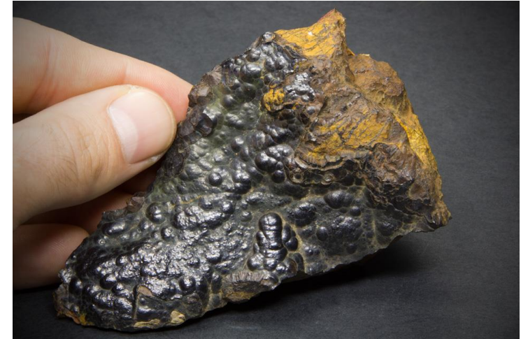
Limonit (barnavasérc) \text{Fe}_2\text{O}_3 \cdot \text{H}_2\text{O} , vastartalom: 30...50%
